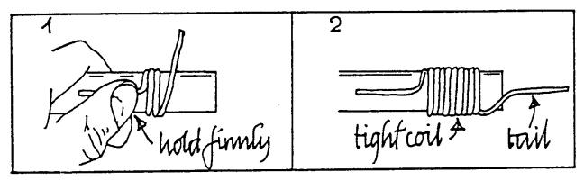
15. Slip the tight coil off the glass tube and adjust the tail so that it bends and then is positioned down the axis of the coil.
